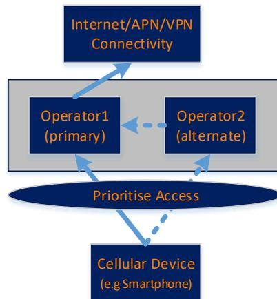
Figure 3b: Access to Multiple RANs (one at a time)
