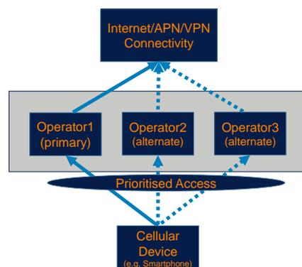
Figure 3a: Access to Multiple RANs (one at a time)
