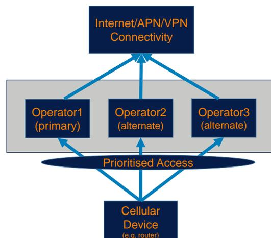
Figure 2: Access to Multiple RANs (simultaneously)
